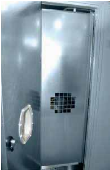
Drive guard (wire mesh)
