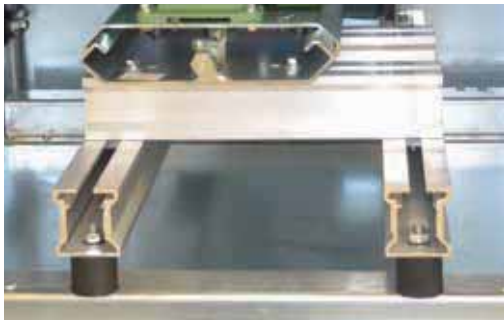
Rubber anti vibration mounts
