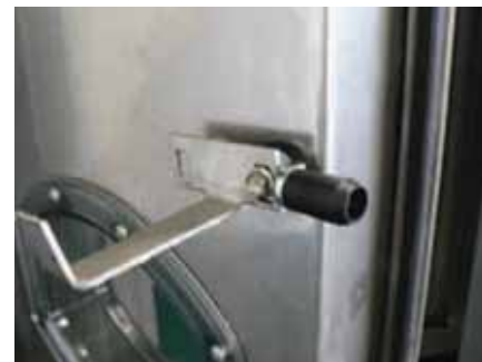
Door high pressure protection (pressure guard)
